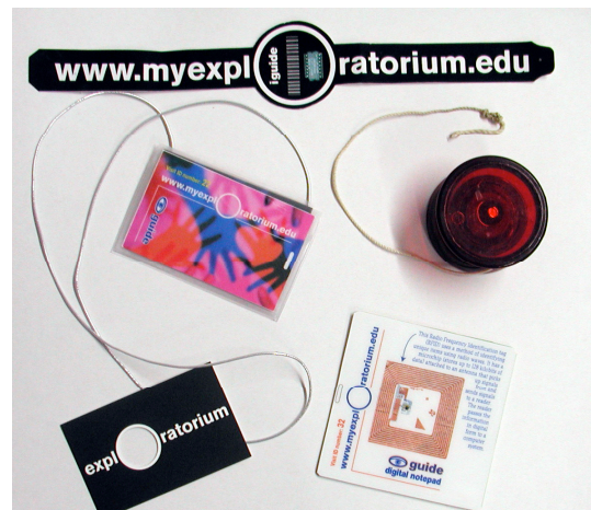
Figure 2: Prototypes for RFID tokens: yo-yo, cards, table coaster, necklace, and watch.
