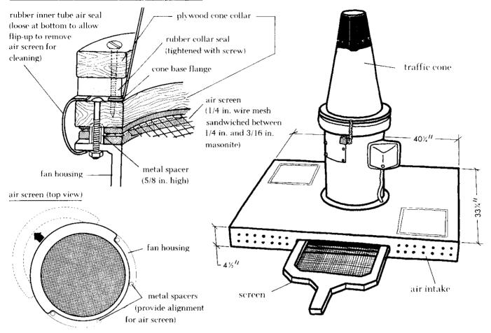
base have been repeatedly drilled through to allow air to get to the fan. A screen accessible from the edge of the base prevents large objects from being sucked up into the fan and expelled at high velocities at people above.
