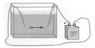
Fill the container with water and place the wires and pencil lead in it so that the pencil lead is positioned horizontally. Connect the two wires to the terminals of the battery, and allow the heating to start. Shine the projector through the liquid, projecting the light onto the screen or white posterboard.
